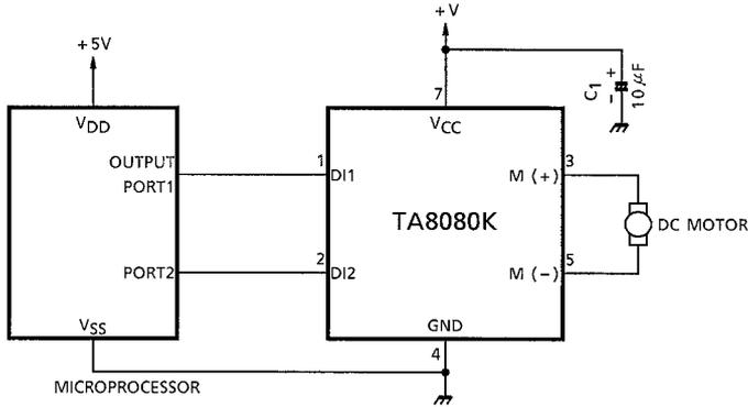
Cautions for Wiring : C<sub>1</sub> is for absorbing disturbance, noise etc.
